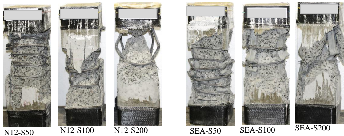
Figure 2 Failure modes of the tested specimens
